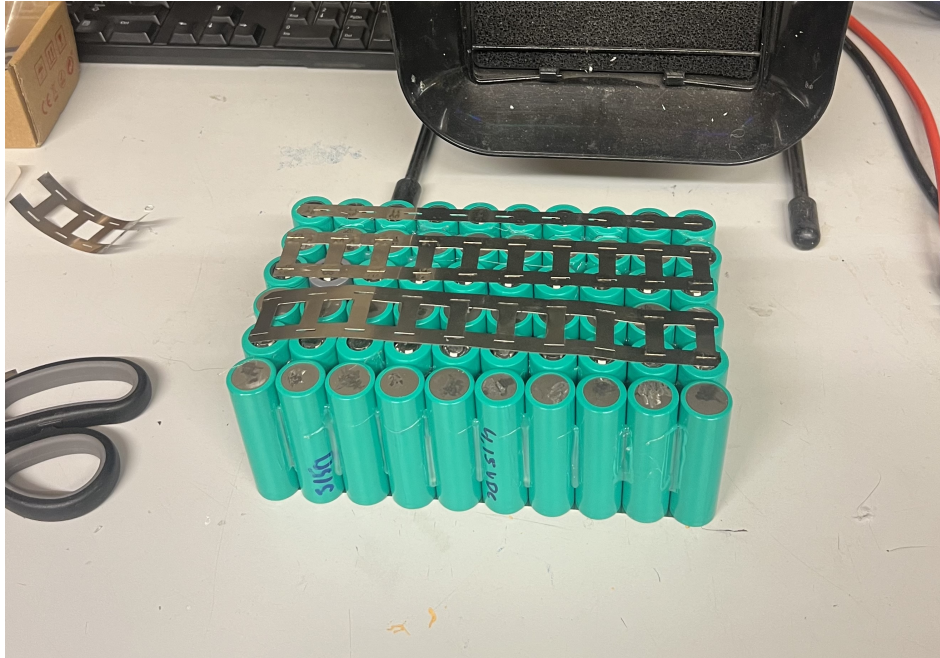
Figure 11: LIION-Battery during assembly
